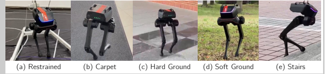
Fig. 6: Reality experiments for P1 conducted on different terrains, adopting AnyBipe ’s best policy.
